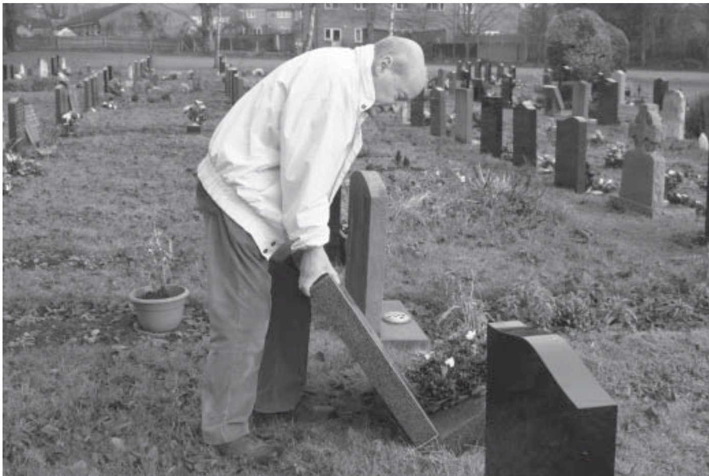
Mike Gee tests the stability of a gravestone, checks found that 79 were loose and four were very unstable.
